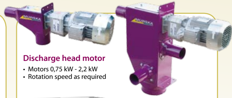
1+2 Discharge head motor • Where spiral conveyors meet • Positions for detectors • Motors 0,75 kW - 2,2 kW • Rotation speed as required
